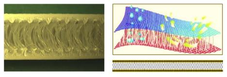
Cross-sectional view and schematic representation of spacer fabric of IPC membrane (Doyen et al., 2008)
