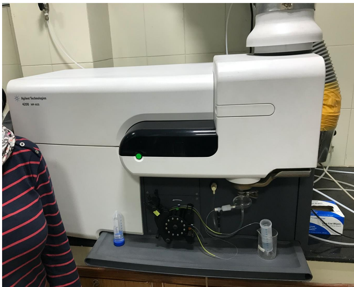
Figure 5: Microwave plasma - atomic emission spectrometry (Agilent MP-AES 4200) at the IIT
