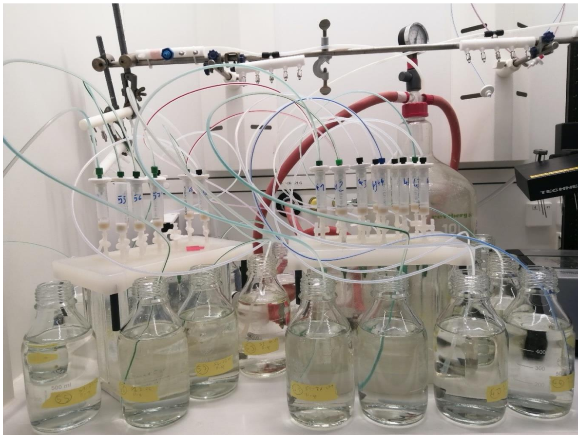
Figure 2: Solid-phase extraction set up with attached cartridges during sample
