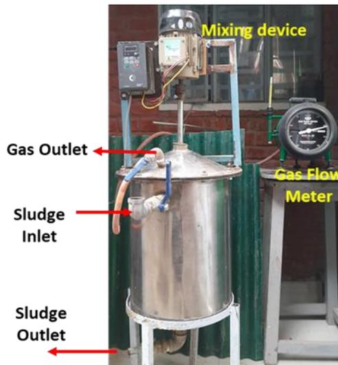
Figure 2-2: Laboratory-scale sludge digestion unit
