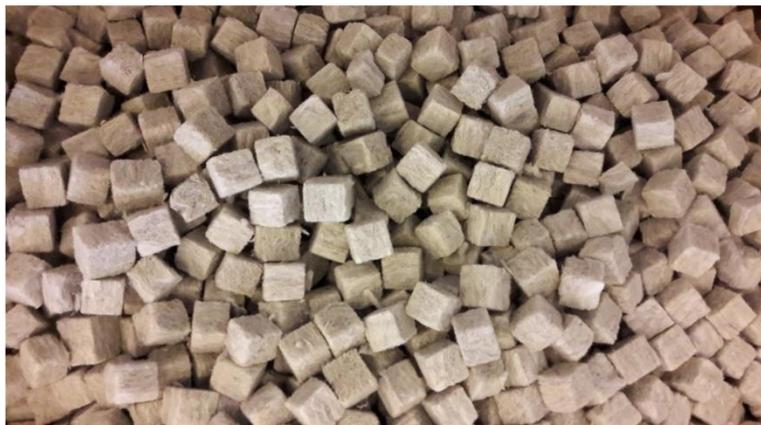
Figure 4-1: Cleanblocks material, made from mineral wool. The cubes shown in this image are around 1 cm<sup>3</sup>.
