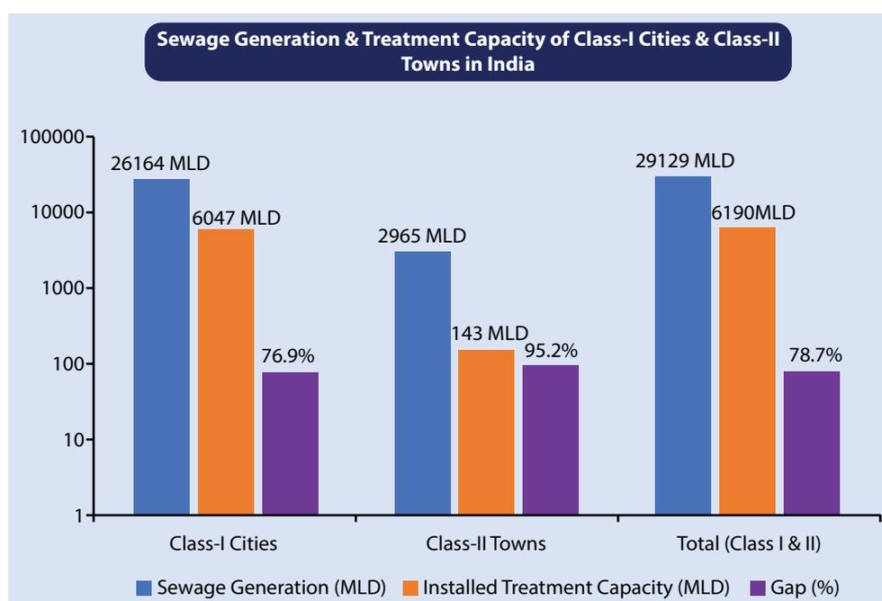
**Figure 1:** Sewage generation and treatment scenario of Class-I cities & Class-II towns of India (log-scale with % gap in treatment)
